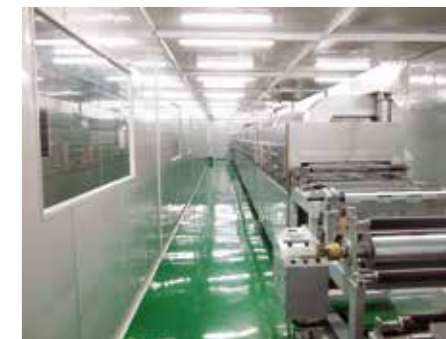
非氟离子传导膜生产线 Produce line of Non-fluoride ion conducting membrane
